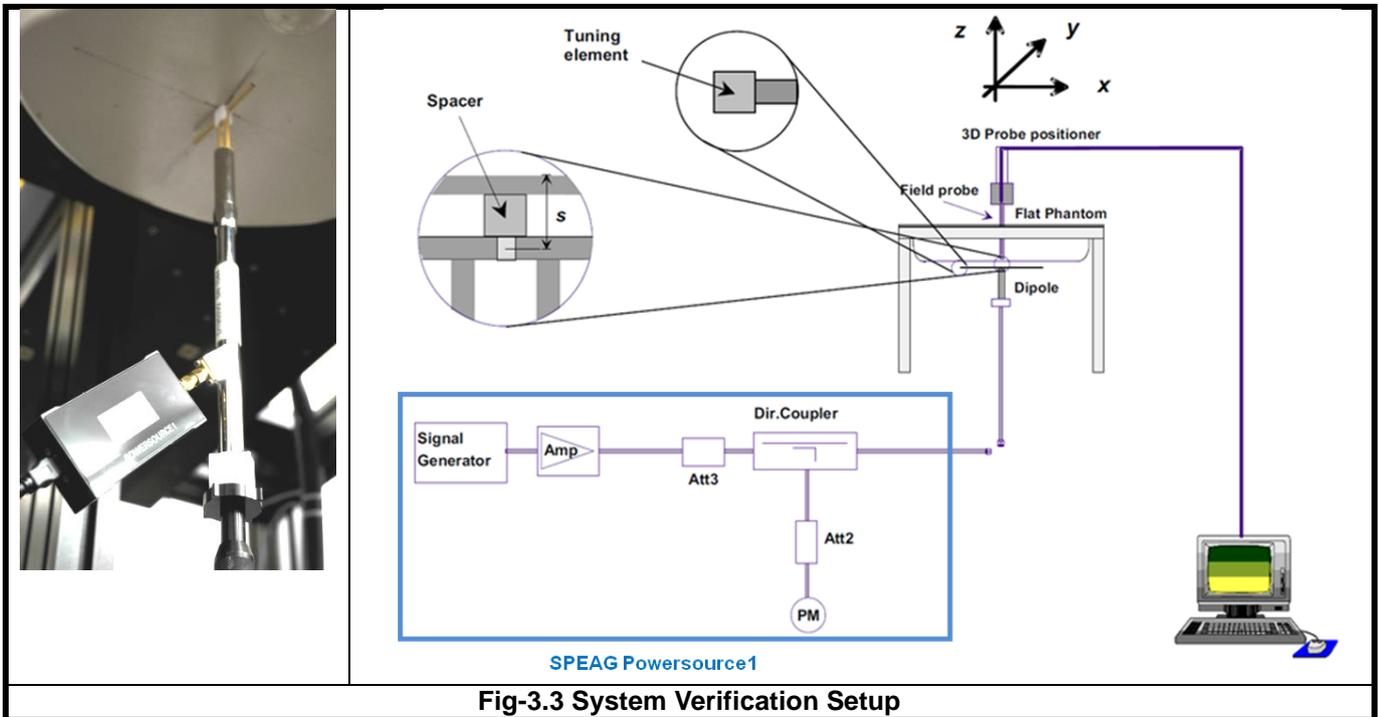
**Fig-3.3 System Verification Setup**
