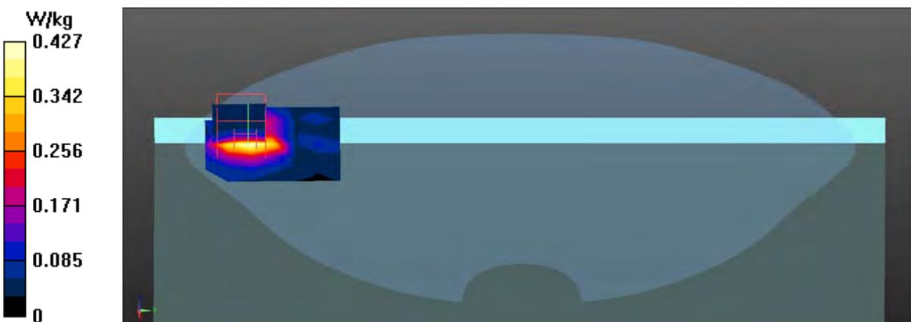
802.11ac80 EUT Top (PAD) (SPEED Main Antenna), Z-Axis plot
