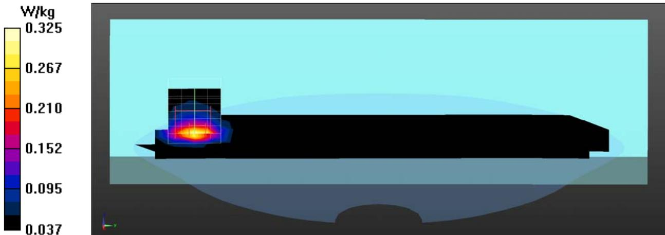
802.11b EUT Back(PAD)(Aux Antenna) Z-Axis plot
