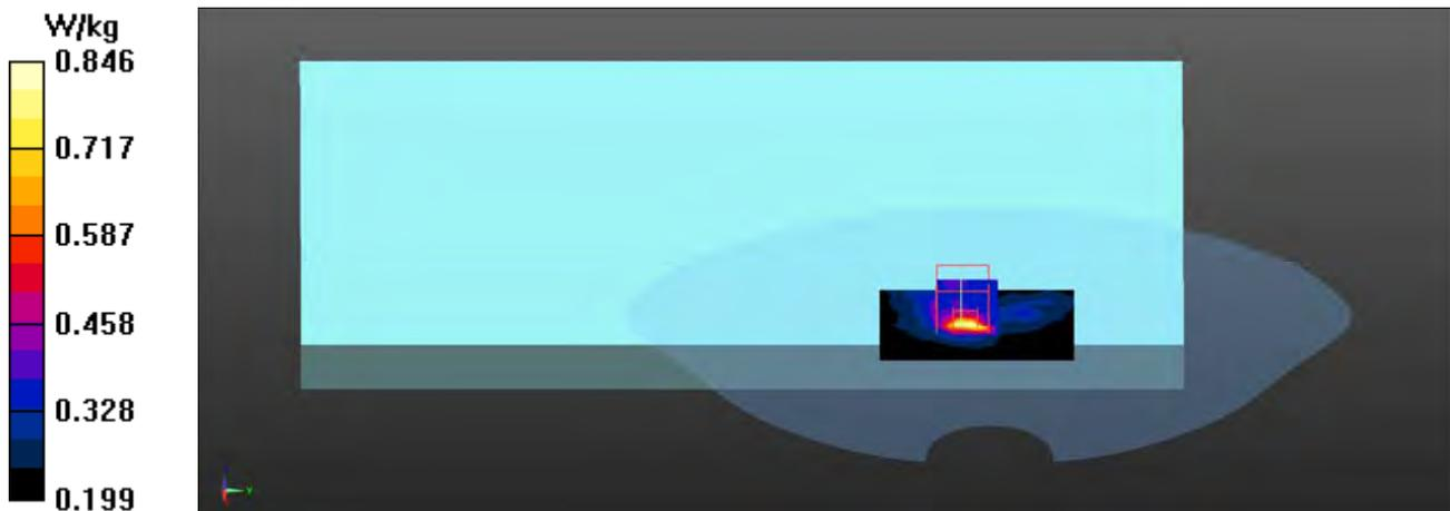
**802.11ac80M EUT Back PAD Mode (INPAQ Main Antenna), Z-Axis plot**
