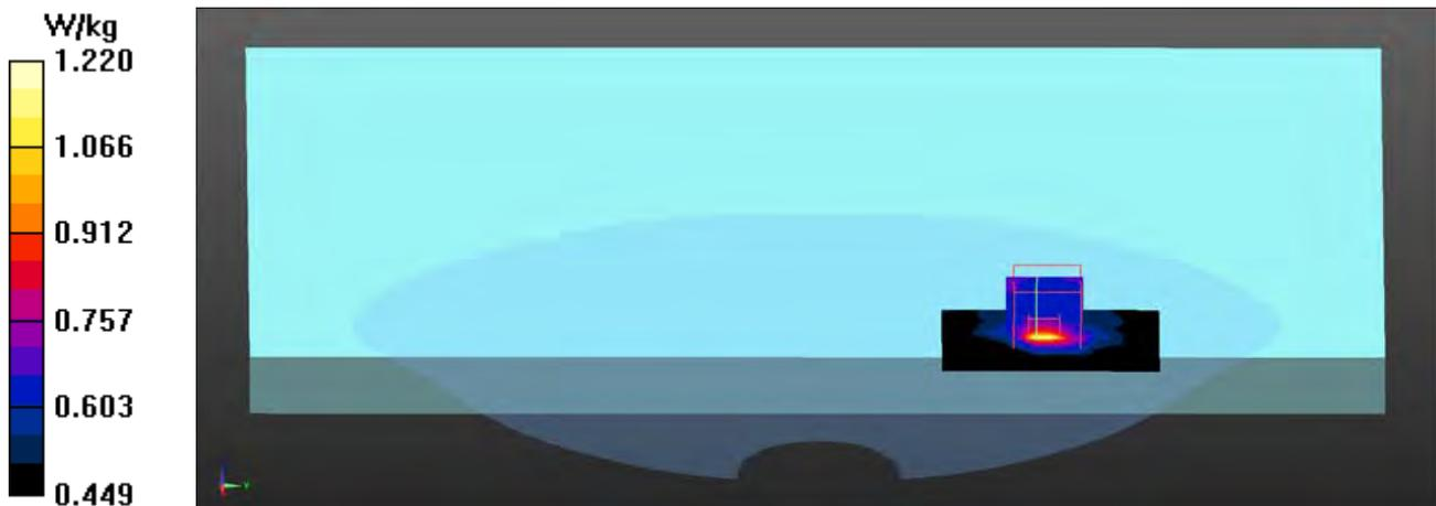
**802.11ac (80M) EUT Back(PAD) (LUXSHARE Main Antenna), Z-Axis plot**
