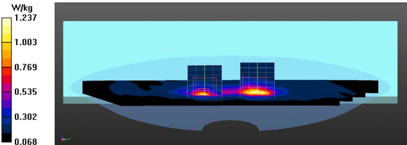
**802.11b EUT Bottom (INPAQ Aux Antenna) Z-Axis plot**
