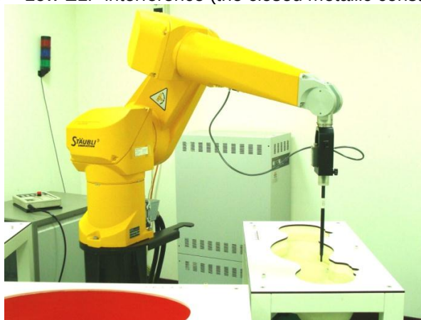
Fig 5.1 Photo of DASY4
