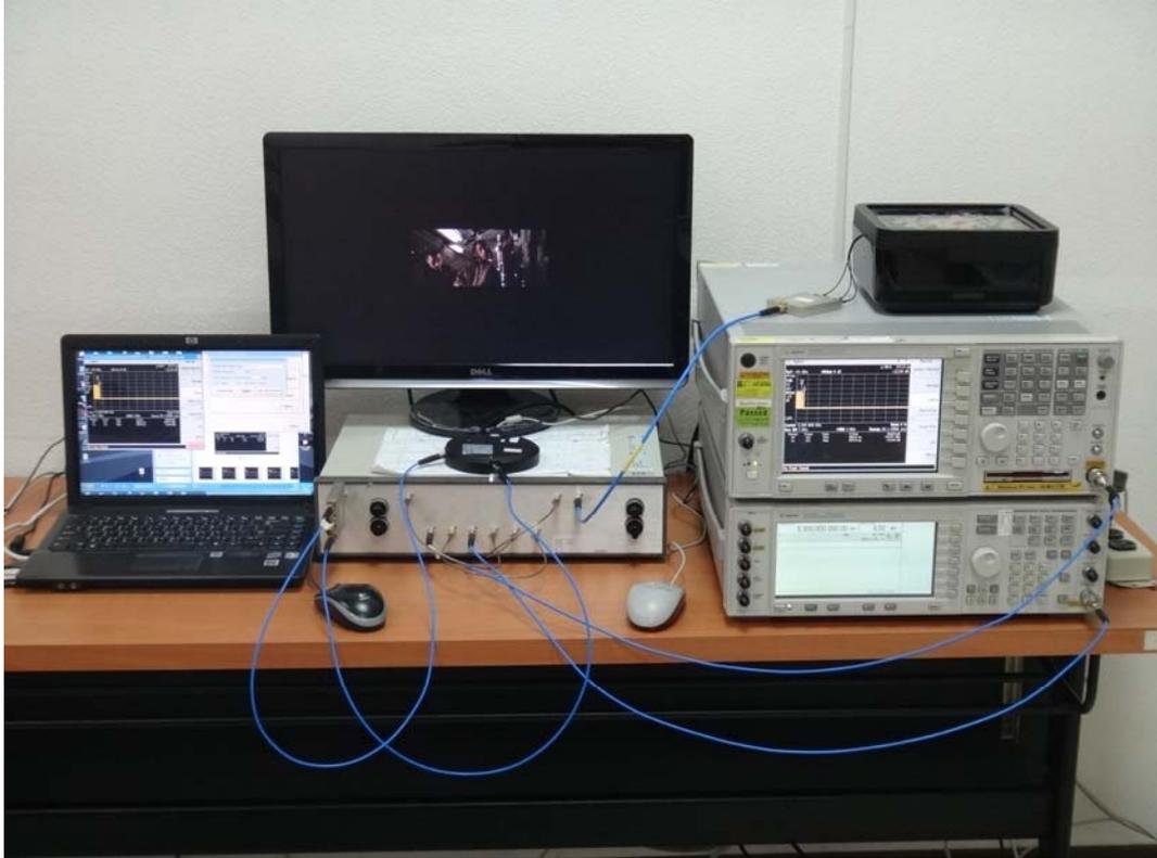
**DFS Set-up Photo: Master and Slave(UUT)**
