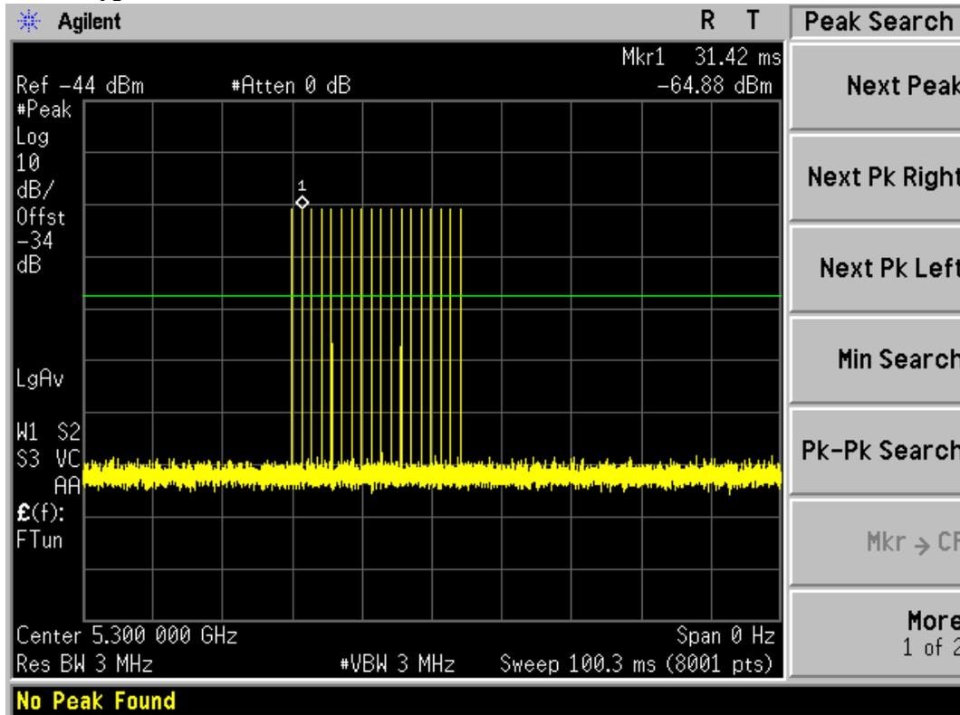
**Radar Type 5 Calibration Plot (5300MHz)**
