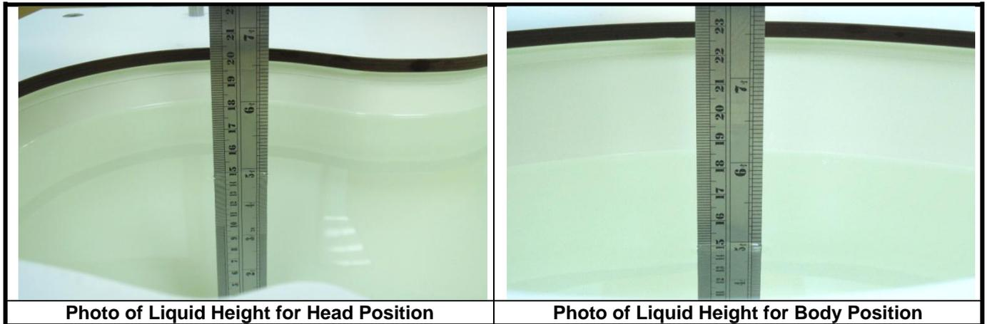
The dielectric properties of the head tissue simulating liquids are defined in IEEE 1528, and KDB 865664 D01 Appendix A. For the body tissue simulating liquids, the dielectric properties are defined in KDB 865664 D01 Appendix A. The dielectric properties of the tissue simulating liquids were verified prior to the SAR evaluation using an Agilent 85070D Dielectric Probe Kit and an Agilent Network Analyzer.
