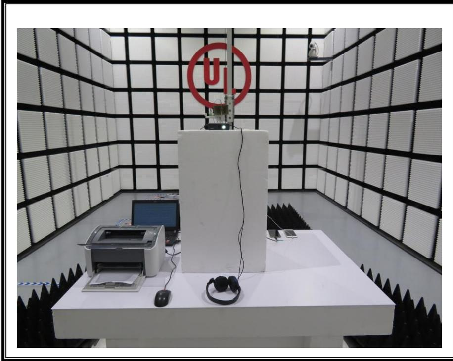
RADIATED RD MEASUREMENT SETUP (30MHz~1GHz)
