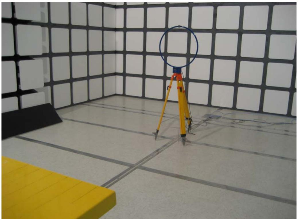
Test Configuration: 30MHz~1GHz
