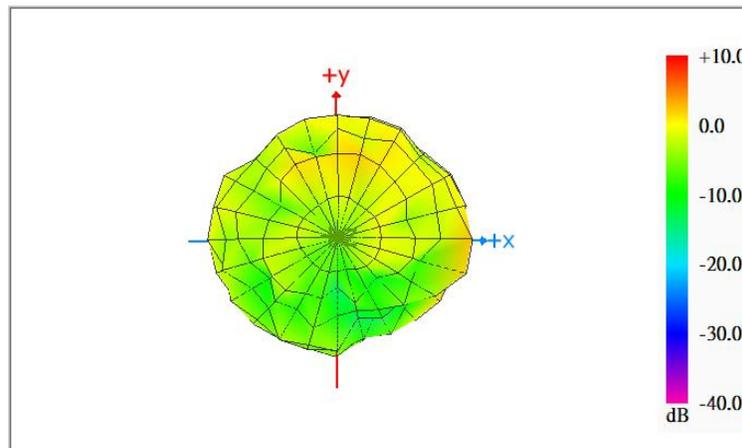
Max Antenna 3D Radiation Pattern 5150-5250 MHz
