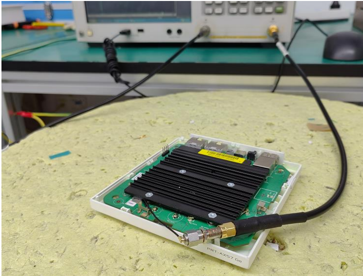
Return loss / Isolation test
