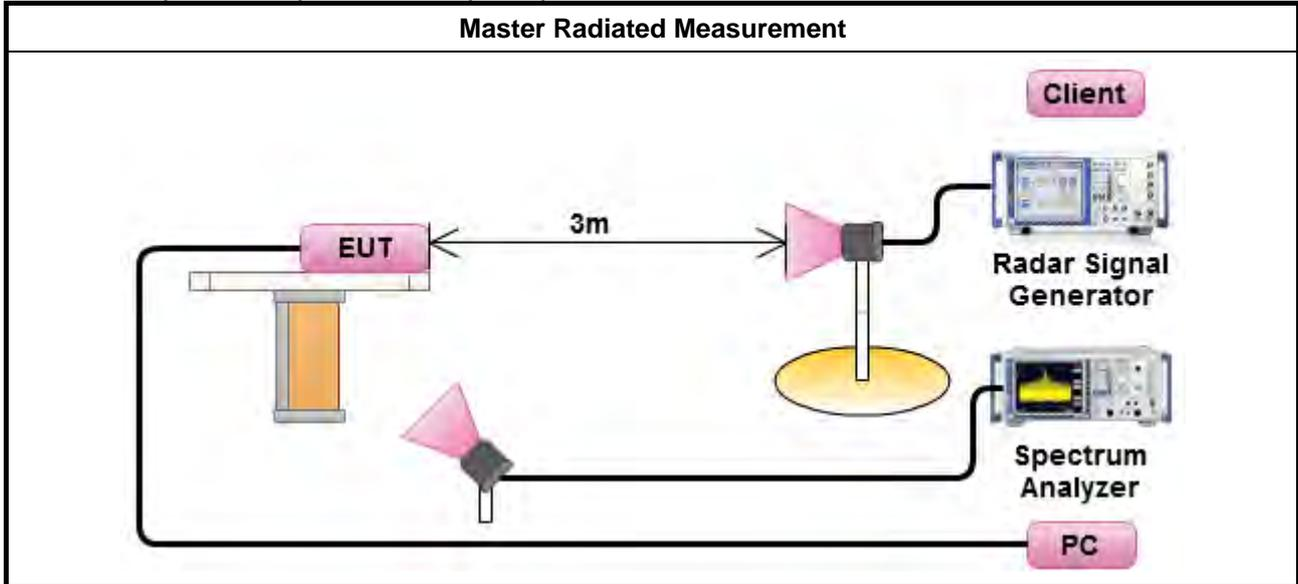
**For Client without radar detection (Bridge):**
