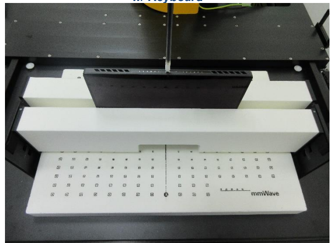
Testing Setup for Power Density, Top Side at 0 mm, w/ Keyboard
