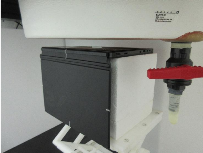
Testing Setup for Body, Back of Display Screen at 25 mm, w/ Keyboard
