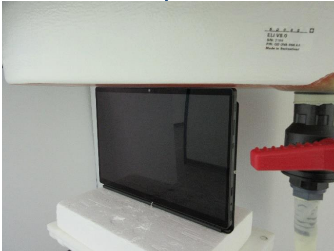
Testing Setup for Body, Top Side at 0 mm, w/ Keyboard
