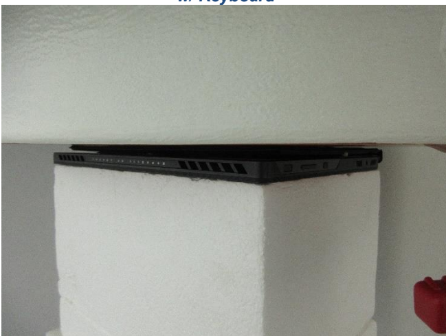
Testing Setup for Body, Bottom Surface at 0 mm, w/ Keyboard
