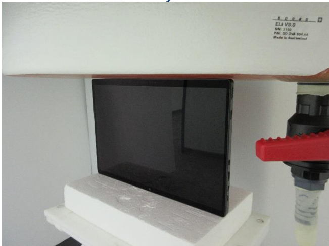
Testing Setup for Body, Bottom Side at 0 mm, w/o Keyboard
