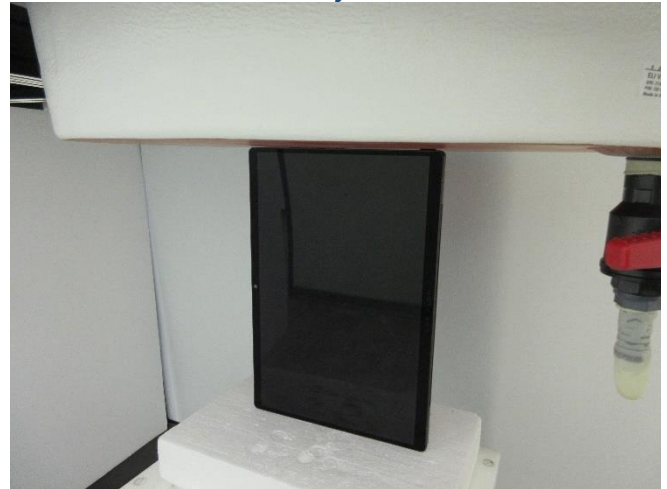
Testing Setup for Body, Right Side at 0 mm, w/o Keyboard
