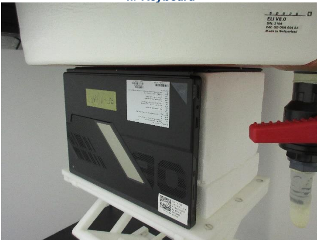
Testing Setup for Body, Bottom of Laptop at 0 mm, w/ Keyboard
