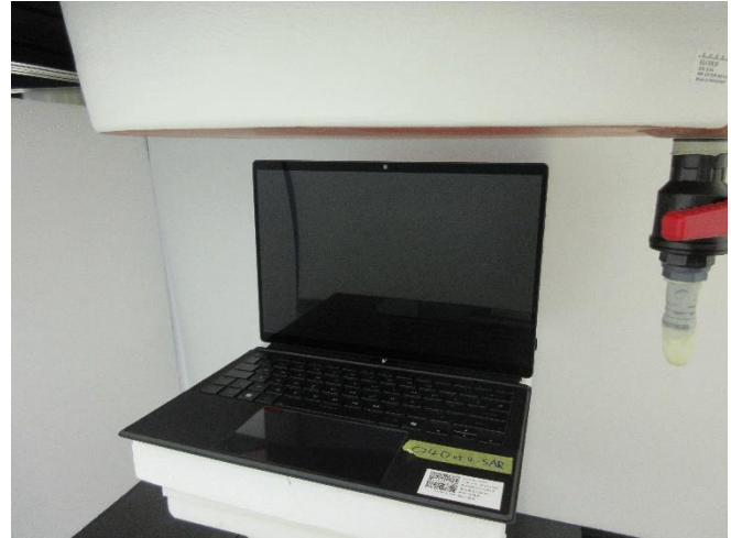
Testing Setup for Body, Top Side of Display Screen at 25 mm, w/ Keyboard
