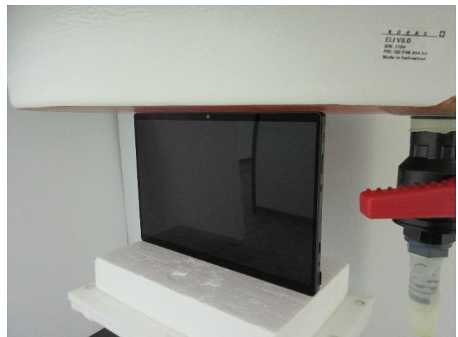
Testing Setup for Body, Top Side at 0 mm, w/o Keyboard
