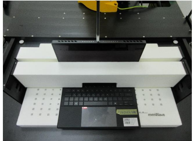
Testing Setup for Power Density, Top Side of Display Screen at 25 mm, w/ Keyboard
