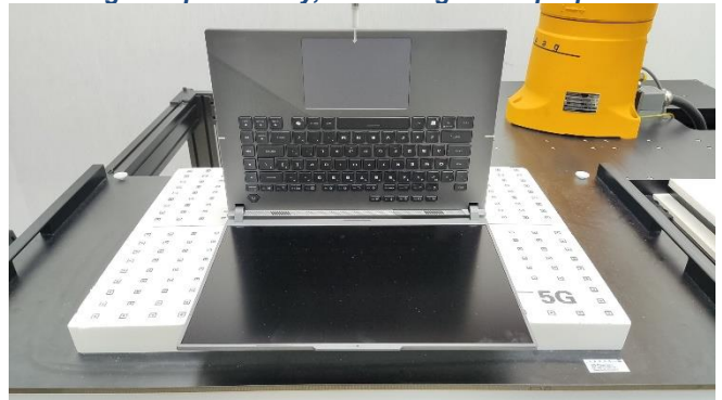
Testing Setup for Body, Front Edge of Laptop at 2 mm
