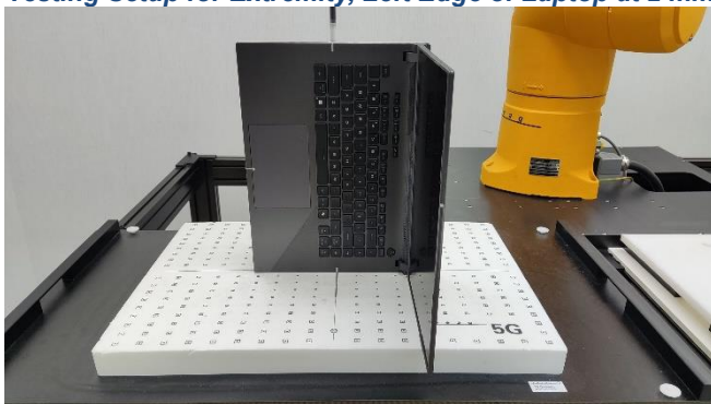
Testing Setup for Extremity, Left Edge of Laptop at 2 mm
