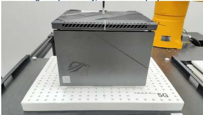
Testing Setup for Body, Bottom of Laptop at 2 mm
