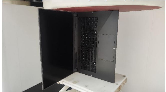
Testing Setup for Extremity, Right Edge of Laptop at 0 mm
