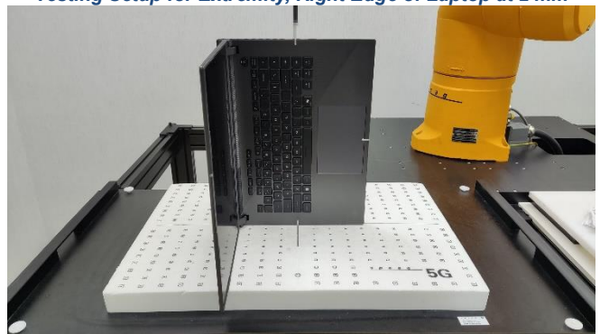
Testing Setup for Extremity, Right Edge of Laptop at 2 mm
