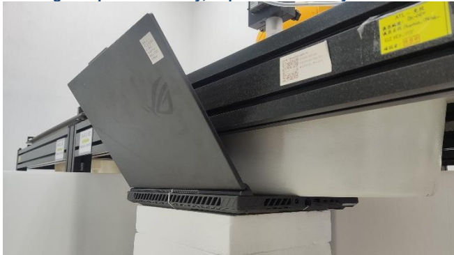
Testing Setup for Extremity, Top Side of the Keyboard at 0 mm
