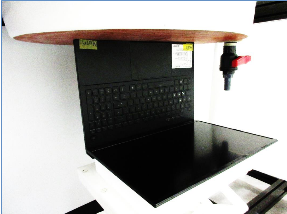
Setup for SAR Testing (Body, Front Edge of Base at 0 mm)
