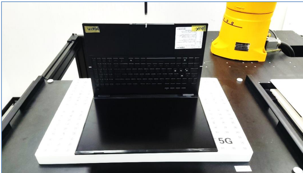
Setup for Power Density Testing (Front Edge of Base at 2 mm)
