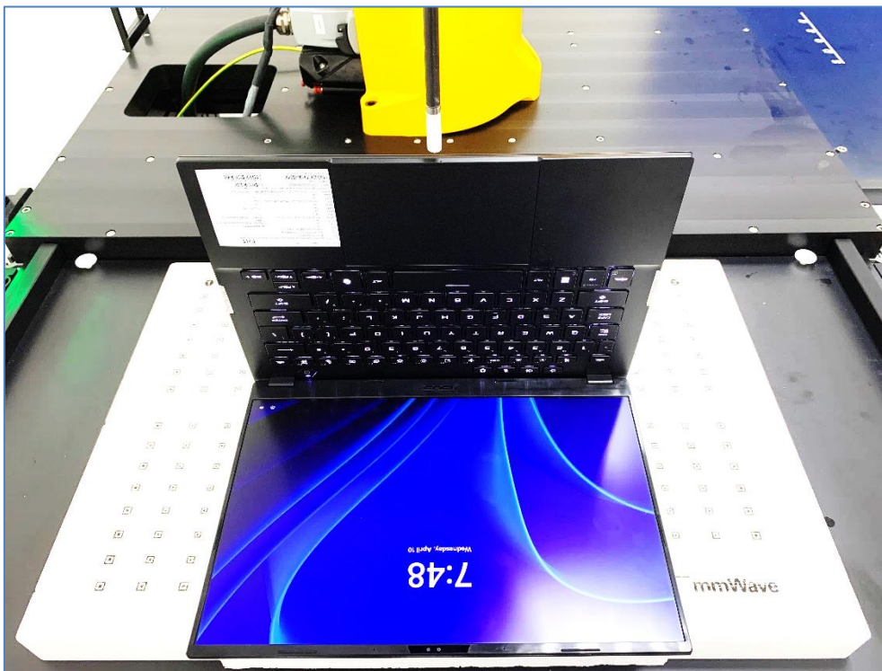
Setup for Power Density Testing (Front Edge of Base at 2 mm)
