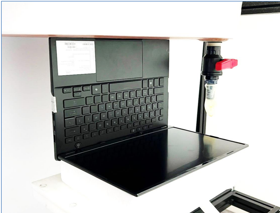
Setup for SAR Testing (Body, Front Edge of Base at 0 mm)
