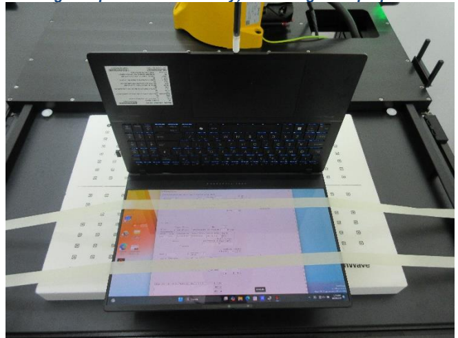
Testing Setup for Power Density, Front Edge of laptop at 0 mm
