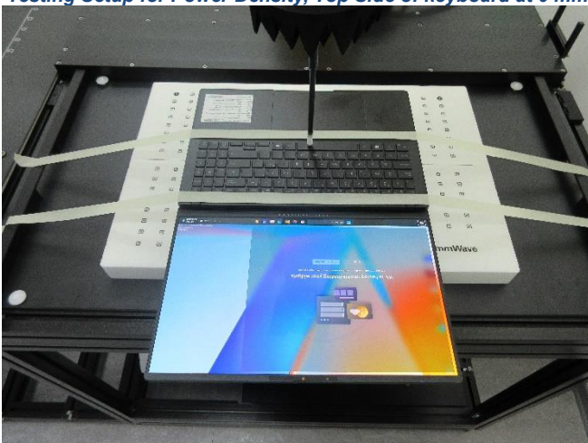
Testing Setup for Power Density, Top Side of keyboard at 0 mm
