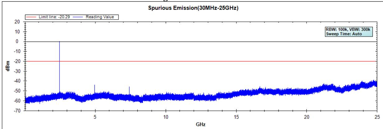
Note: The above test pattern is synthesized by multiple of the frequency range.
