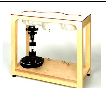
Fig 5.9 Photo of SAM Phantom
