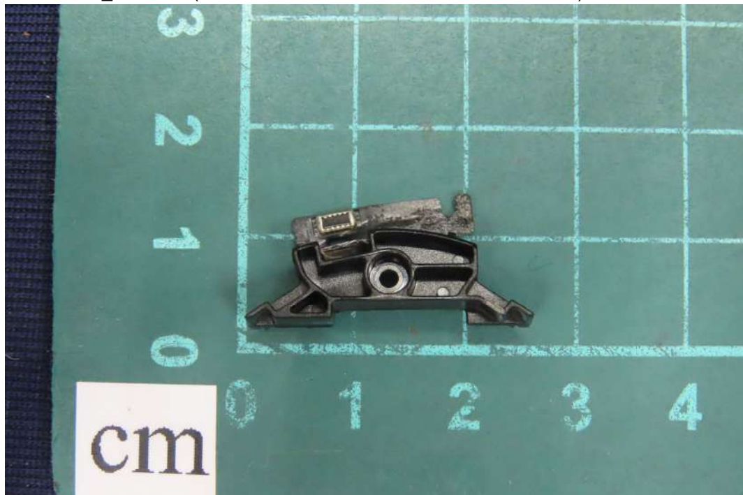
(24) EUT Photo _ Antenna (Brand Name: INPAQ, M/N: WA-C2-LA-00-003)
