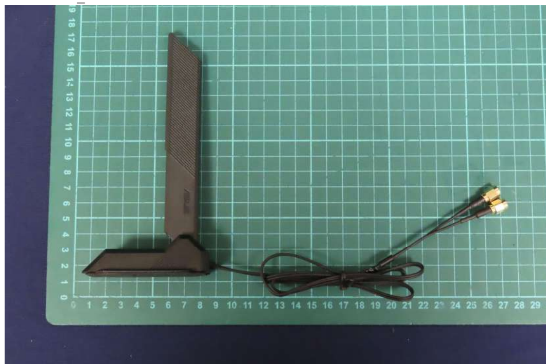
(28) EUT Photo _Wi-Fi & Bluetooth Antenna
