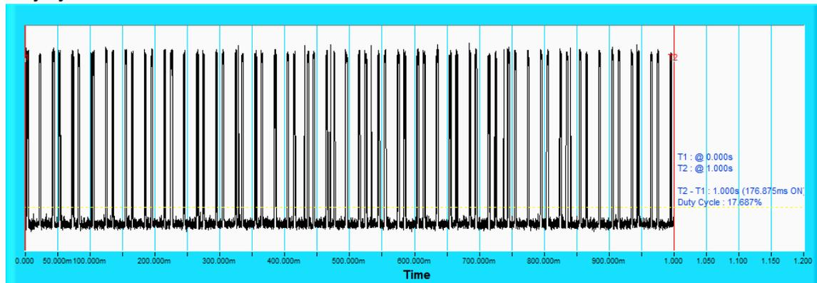
**NOTE:** T1 denotes the start of duty cycle period is 0th second. T2 denotes the end of duty cycle period is 1th second.  $T2 - T1 = 1$  seconds. Duty Cycle = 17.687%.
