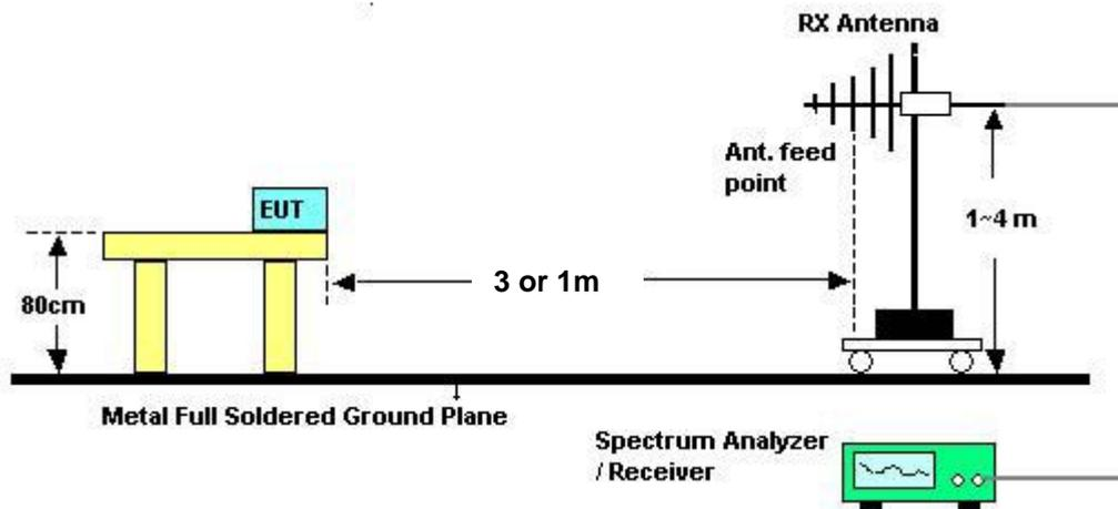
Above 5GHz shall be extrapolated to the specified distance using an extrapolation factor of 20 dB/decade from 3m to 1m.
