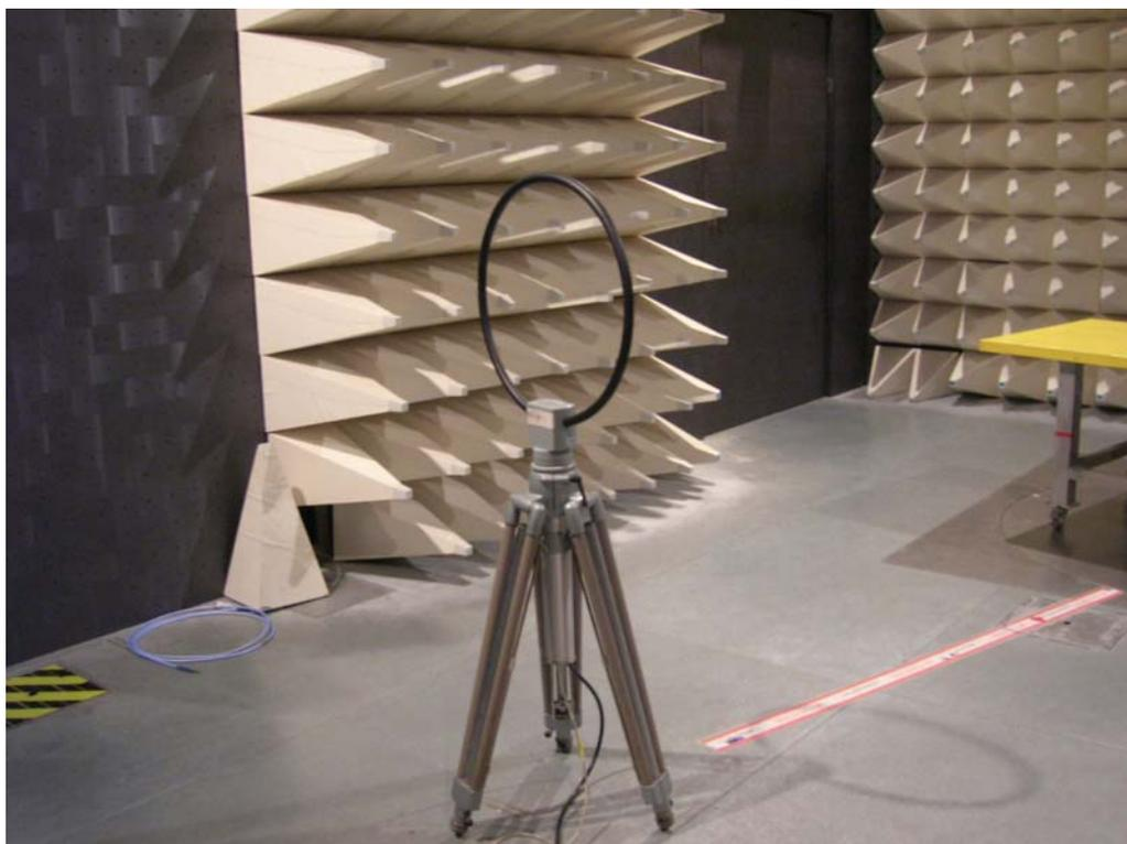
**For radiated emissions 30MHz~1GHz**
