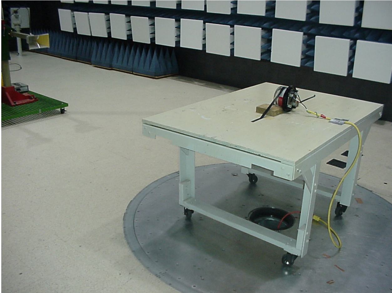
Figure 8 - Radiated Emissions Test Setup (Chamber - Back)
