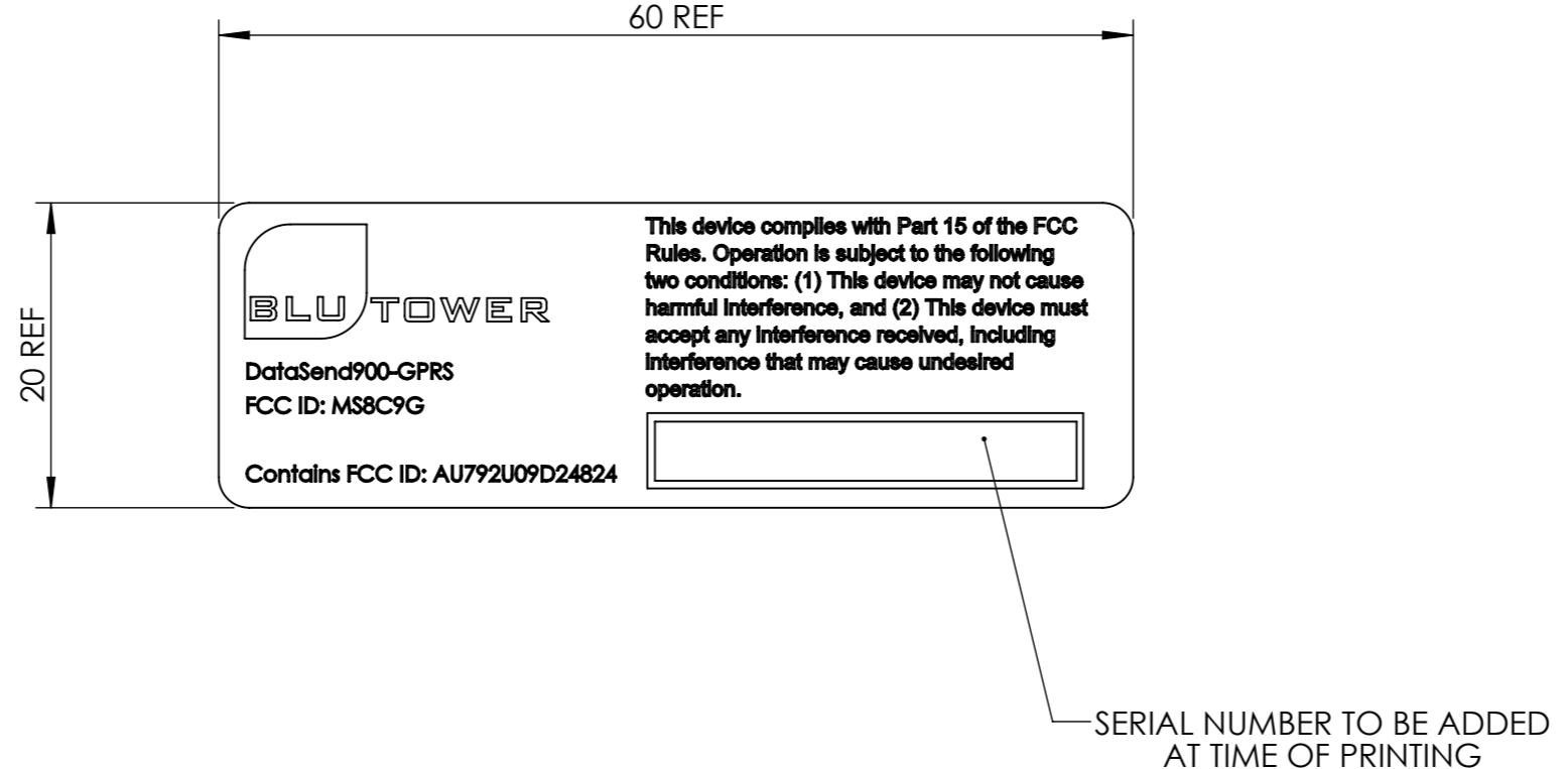
The drawing shows a rectangular label with a black border. Inside, there is a logo for 'BLU TOWER' with a stylized 'U' shape, followed by the text 'DataSend900-GPRS' and 'FCC ID: MS8C9G'. Below this, it says 'Contains FCC ID: AU792U09D24824'. To the right of the text is a small rectangular box with a line pointing to it from the text 'SERIAL NUMBER TO BE ADDED AT TIME OF PRINTING'. Dimension lines indicate a width of 60 REF and a height of 20 REF.
