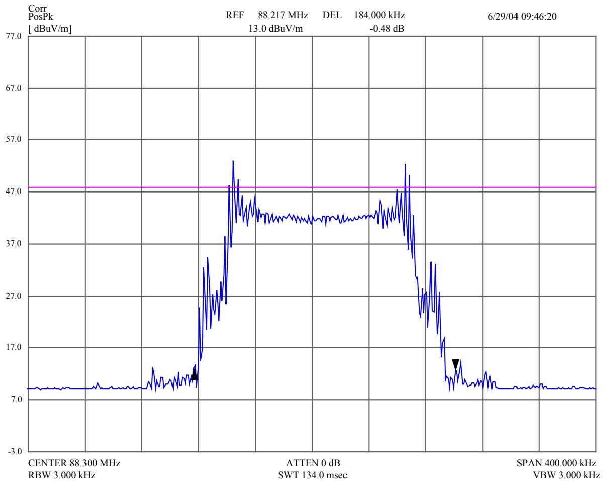
The plot shows the 26 dB bandwidth equals 184 kHz
