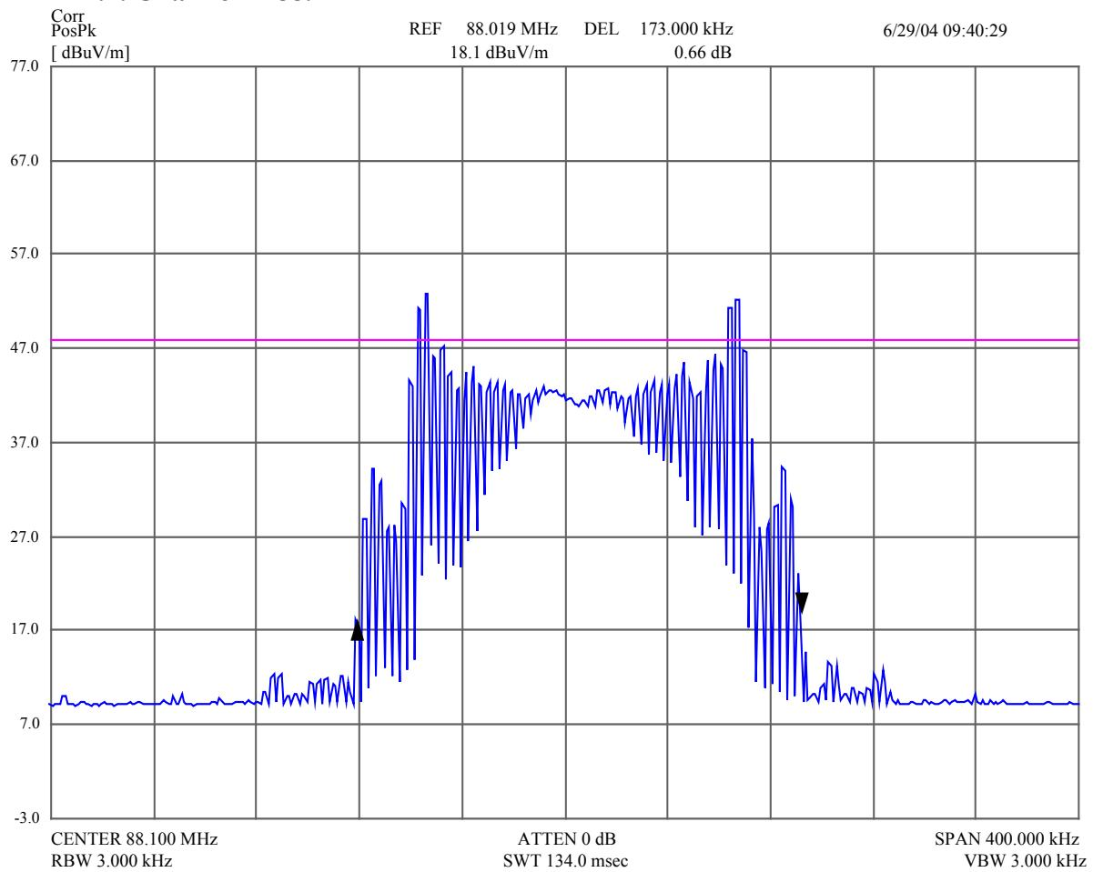
The plot shows the 26 dB bandwidth equals 173 kHz
