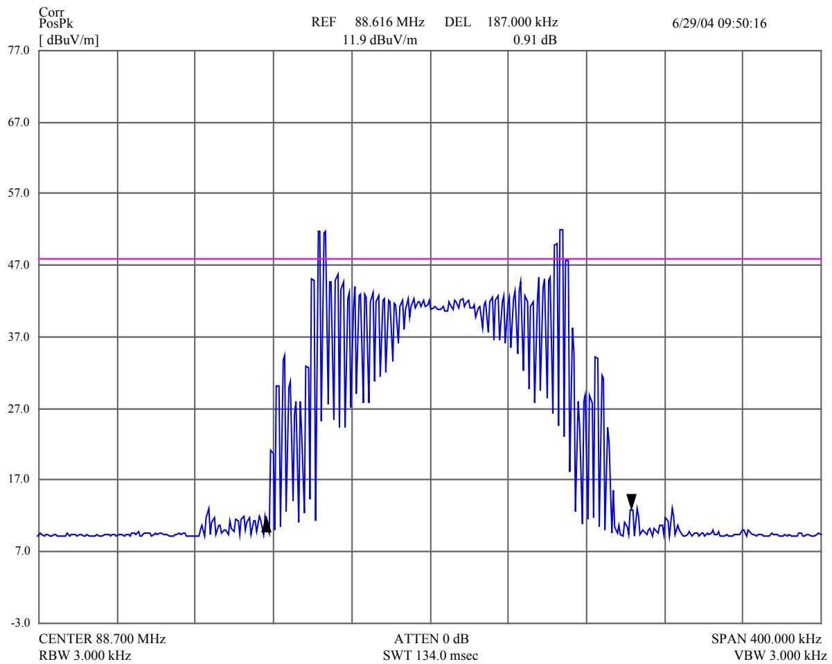
The plot shows the 26 dB bandwidth equals 187 kHz
