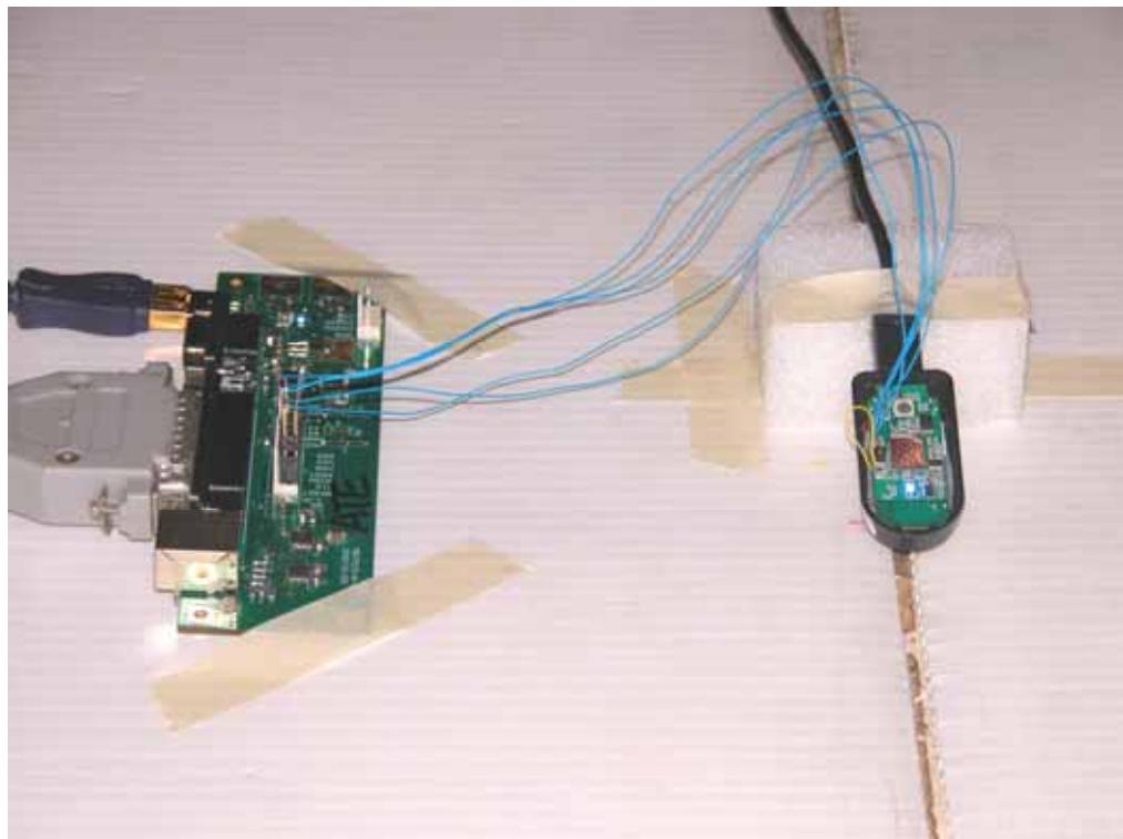
**ANTENNA PORT CONDUCTED RF MEASUREMENT SETUP**
