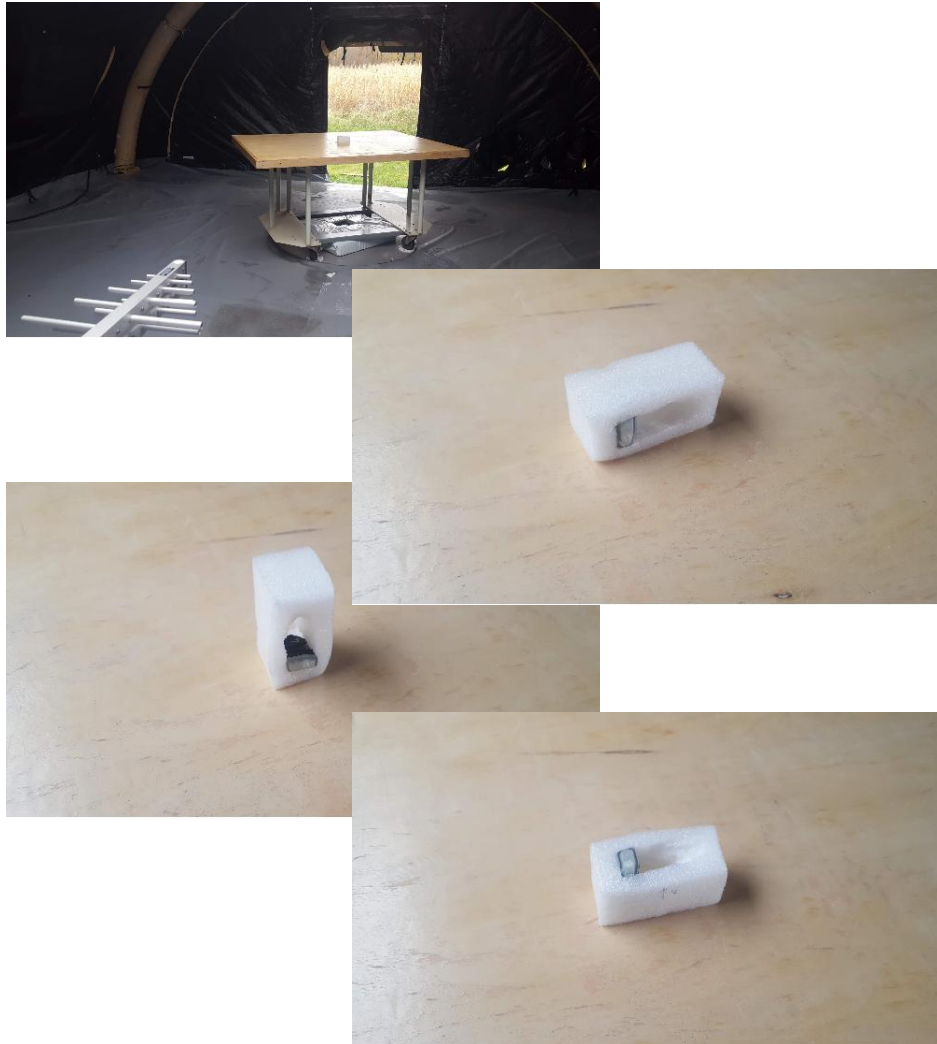
Figure 4: Radiated Emissions Test Setup Photograph(s).
