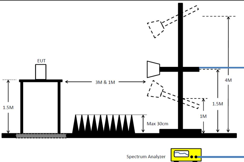
Electric field tests shall be performed in the frequency range of 1 GHz to 10th harmonic of highest fundamental frequency or 40 GHz using a calibrated horn antenna.
