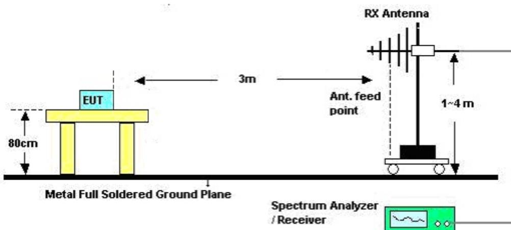
Electric field tests shall be performed in the frequency range of 30 MHz to 1000 MHz using a calibrated bi-log antenna.
