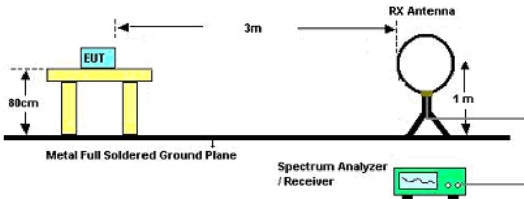
Magnetic field tests shall be performed in the frequency range of 9 kHz to 30 MHz using a calibrated loop antenna.
