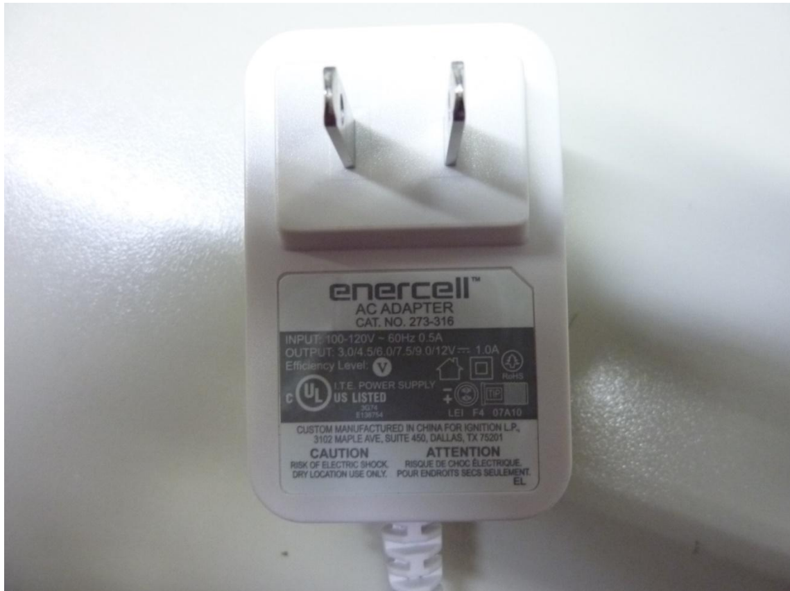
172629_18.jpg: Power supply – type label
