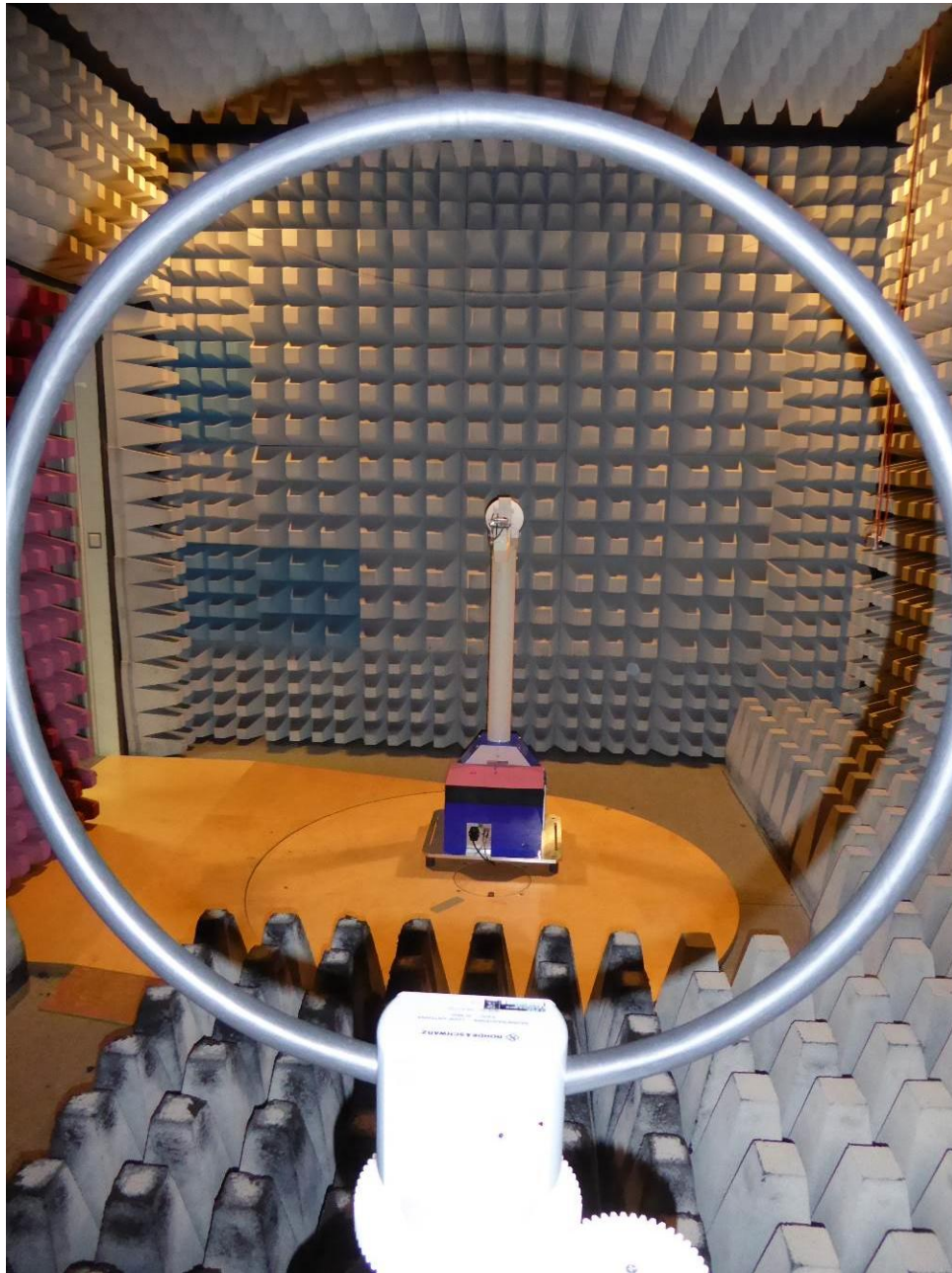
170226_05: Test setup antenna port terminated - Radiated emission anechoic chamber
