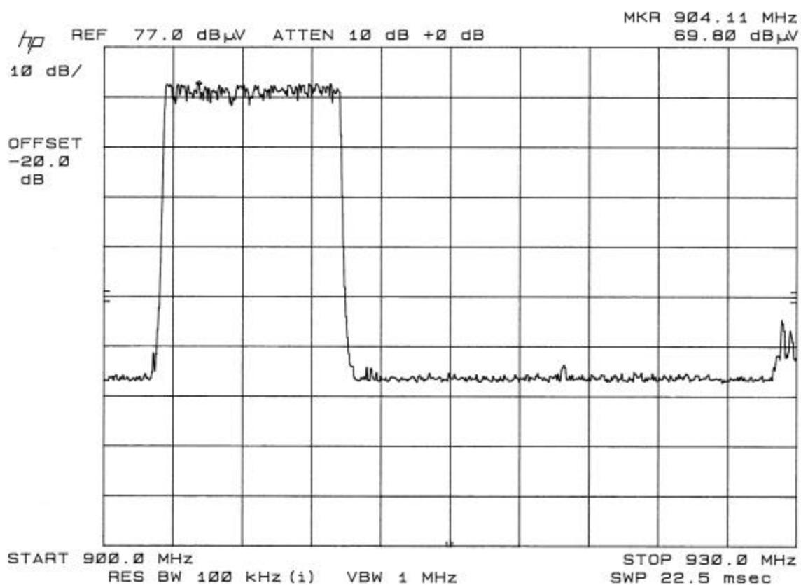
This is a bandedge plot showing both lower bandedge and upper bandedge with the transceiver in hopping mode. There are no significant spurious emissions. The emissions shown at the top of the band are those of paging systems in the 929 to 931 MHz band.
