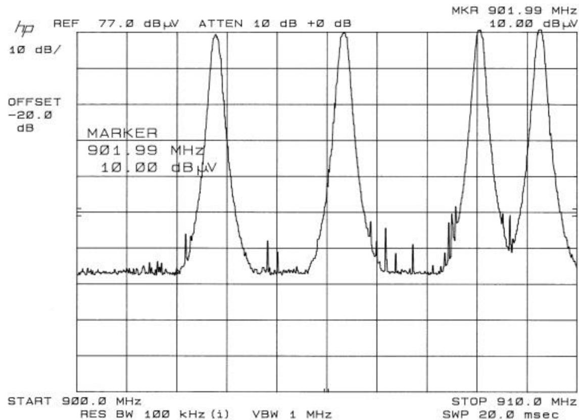
This is a plot of the lower bandedge showing a close in view of several hopping channels and any spurious emissions.
