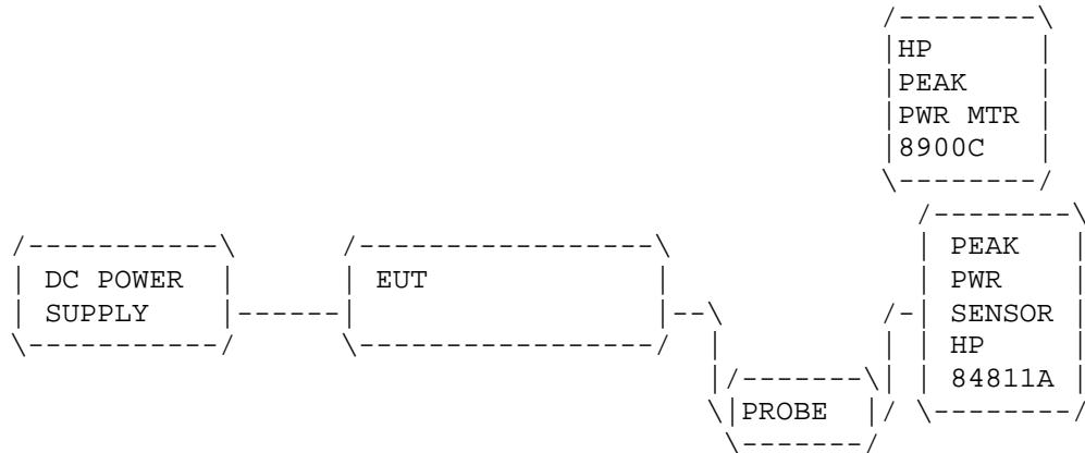
POWER OUTPUT: The RF power output was measured at the antenna feed point by removing the permanent antenna and connecting the UUT to a peak power meter, HP Model No. 8900C.
