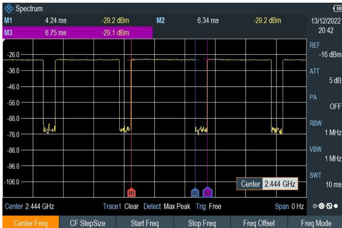
Time-domain plot for Bluetooth transmission signal
