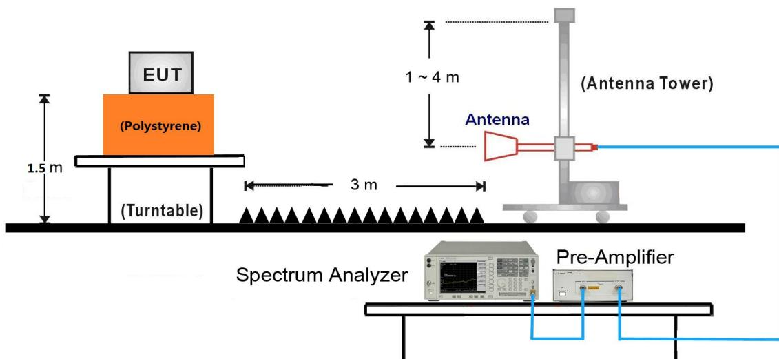
18GHz ~25GHz Test Setup:
