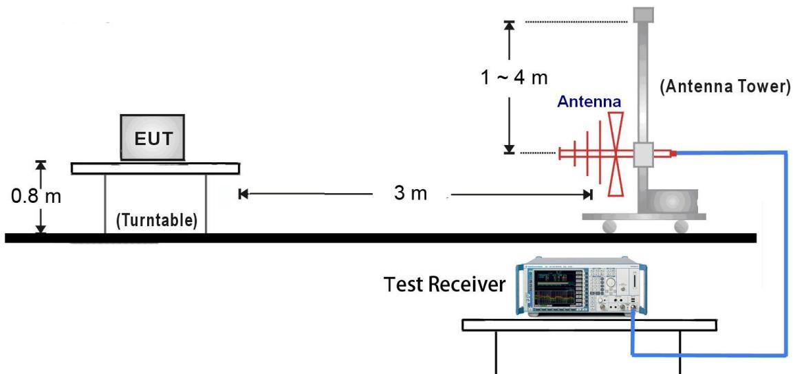
1GHz ~ 18GHz Test Setup:
