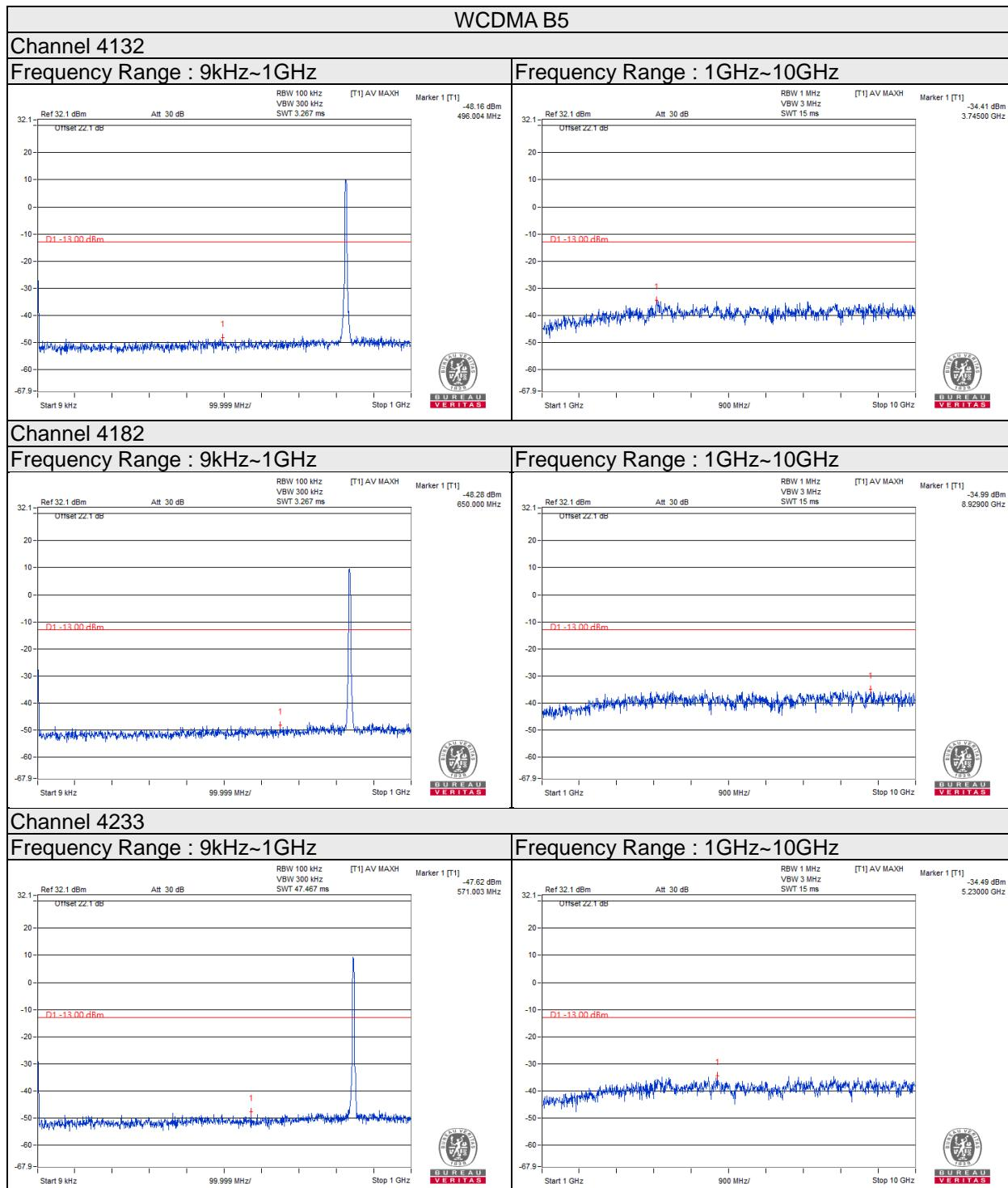
Note: The signal of 9kHz is IF signal from test instrument.
