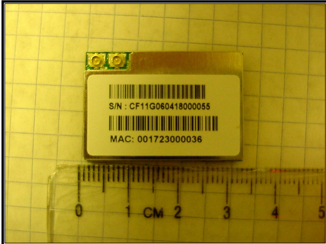
Photograph 15: Radio Top View, With Shield
