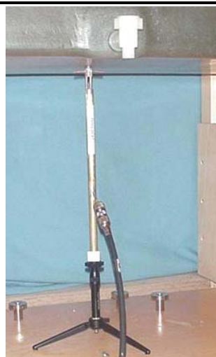
2.4 GHz Validation Dipole Setup
