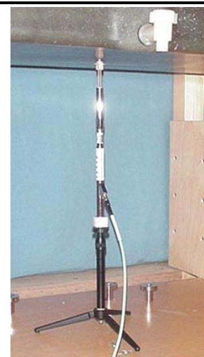
5 GHz Validation Dipole Setup
