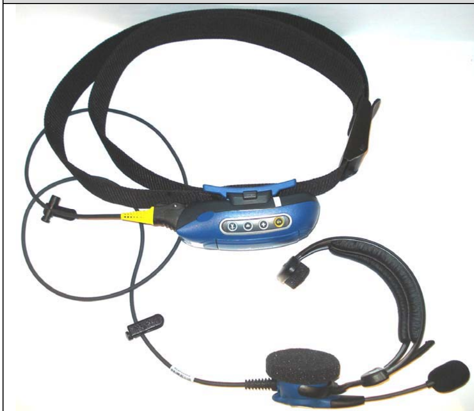
DUT with Headset-Microphone audio accessory & Belt-Clip/Belt-Strap body-worn accessory
