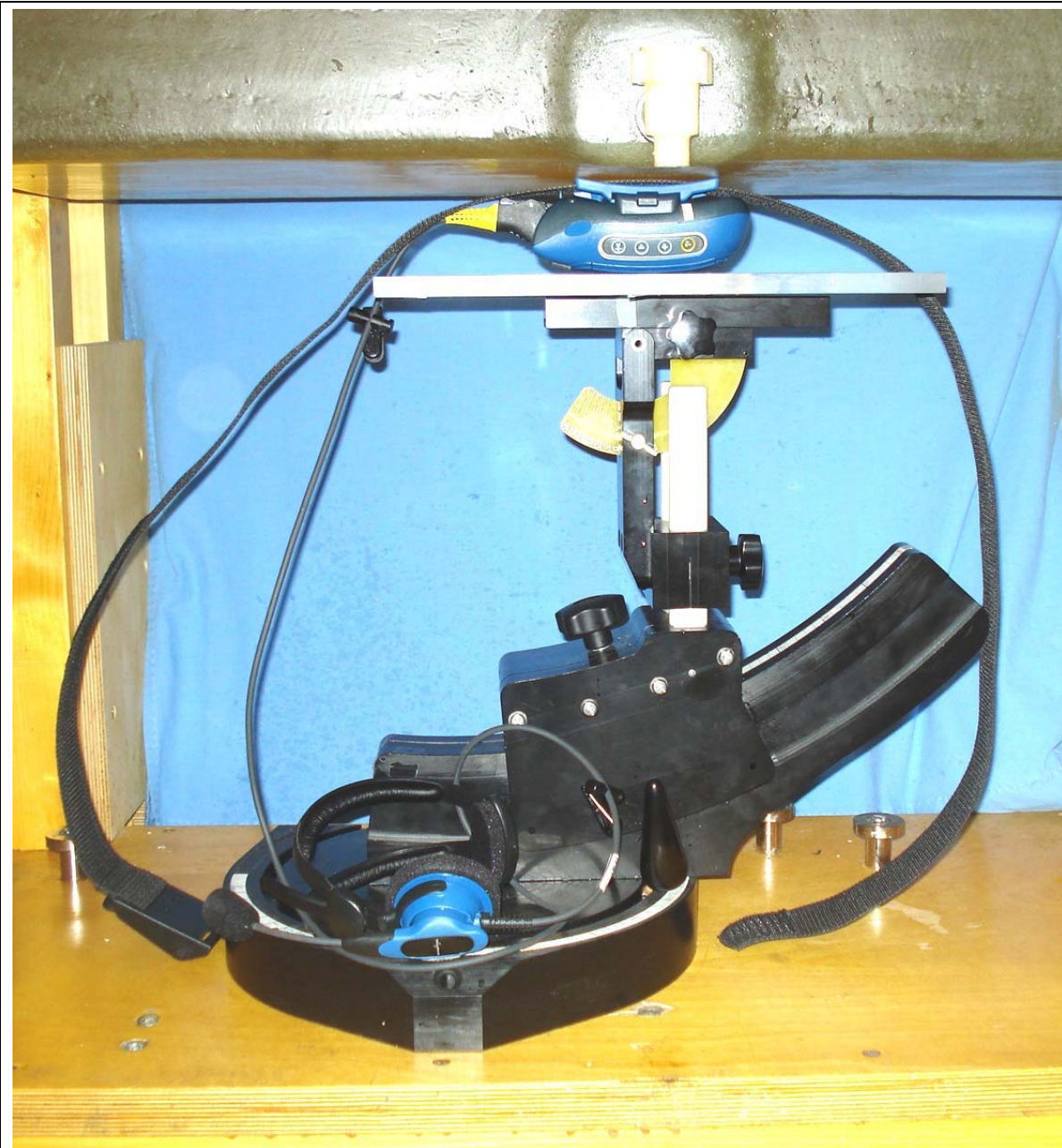
DUT with Belt-Clip/Belt-Strap Body-worn Accessory and Headset-Microphone Audio Accessory
