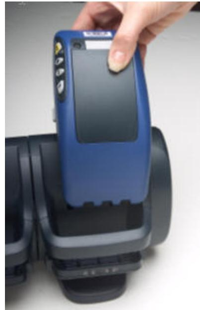
**Figure 5: Inserting a T2 Series Device Into a Charger**
