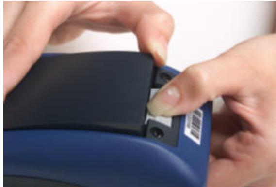
**Figure 29: Removing the Battery From a Device**
