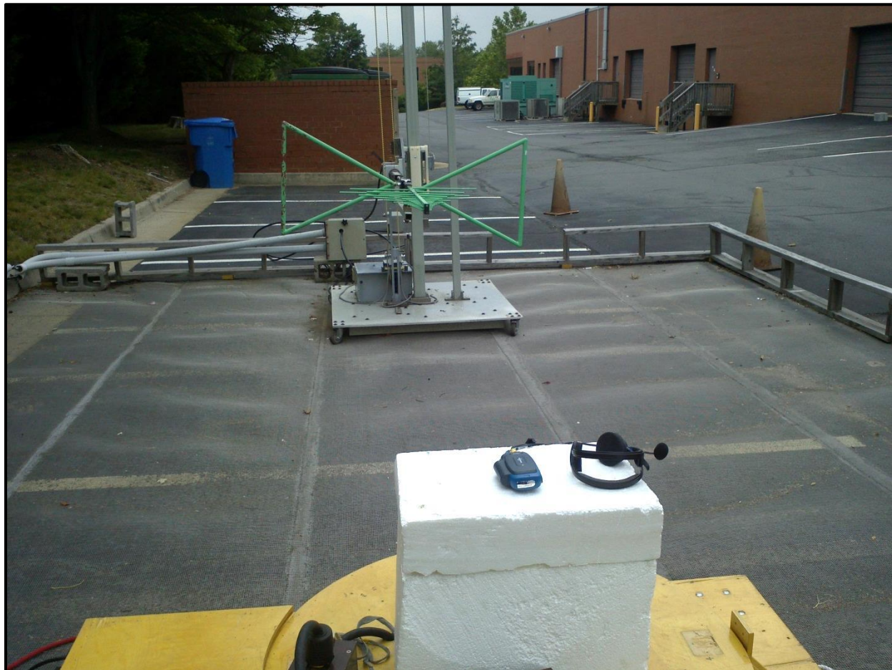
Photograph 1: Unintentional Radiated Emissions Testing – Front View
