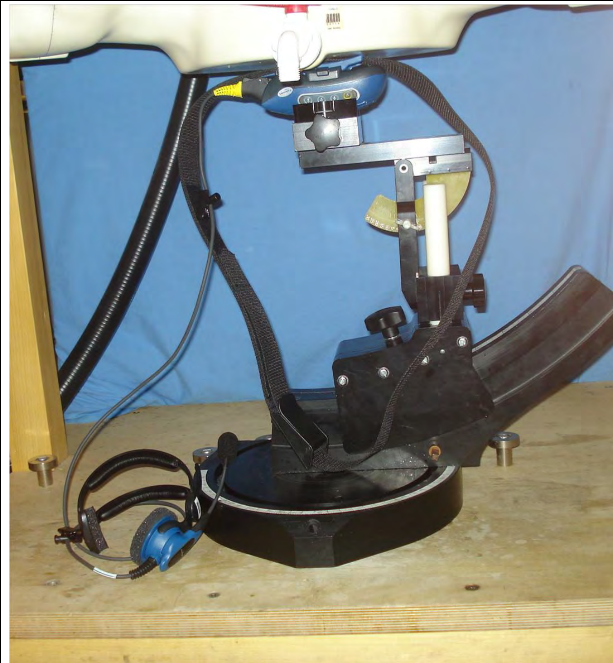
Body-worn Test setup - Belt-clip & Belt-strap Body-worn accessory with Headset-Microphone Audio Accessory
