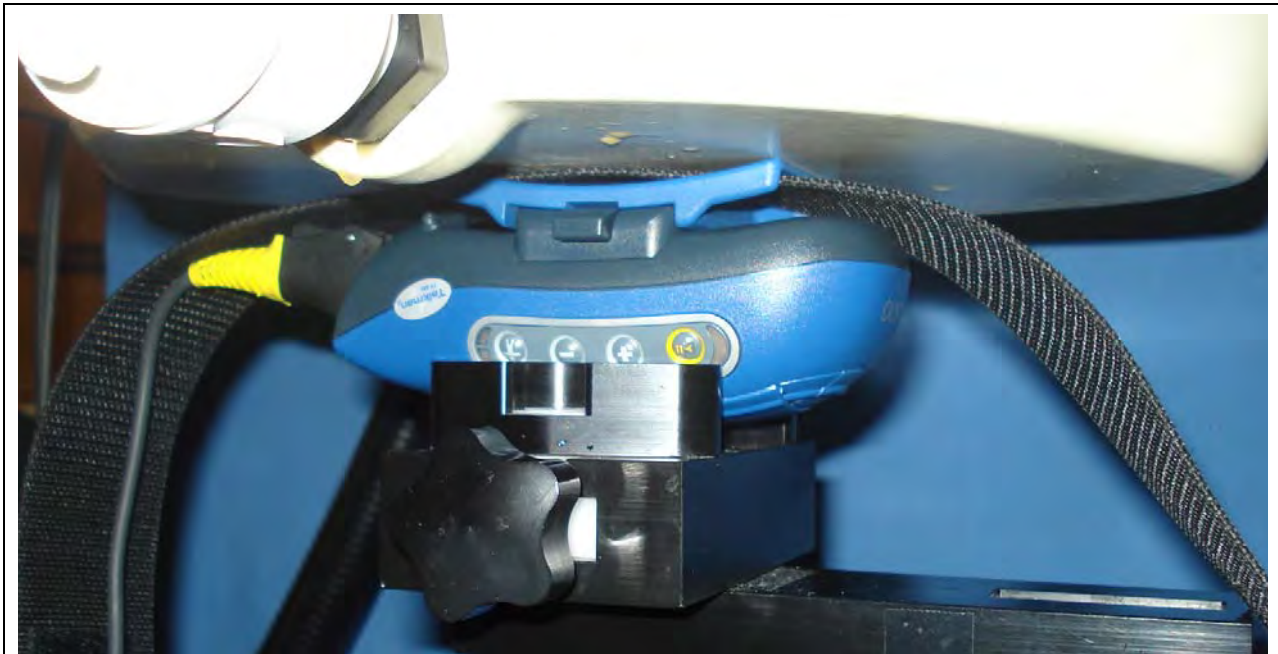
Body-worn Test setup close-up - Belt-clip & Belt-strap Body-worn accessory with Headset-Microphone Audio Accessory
