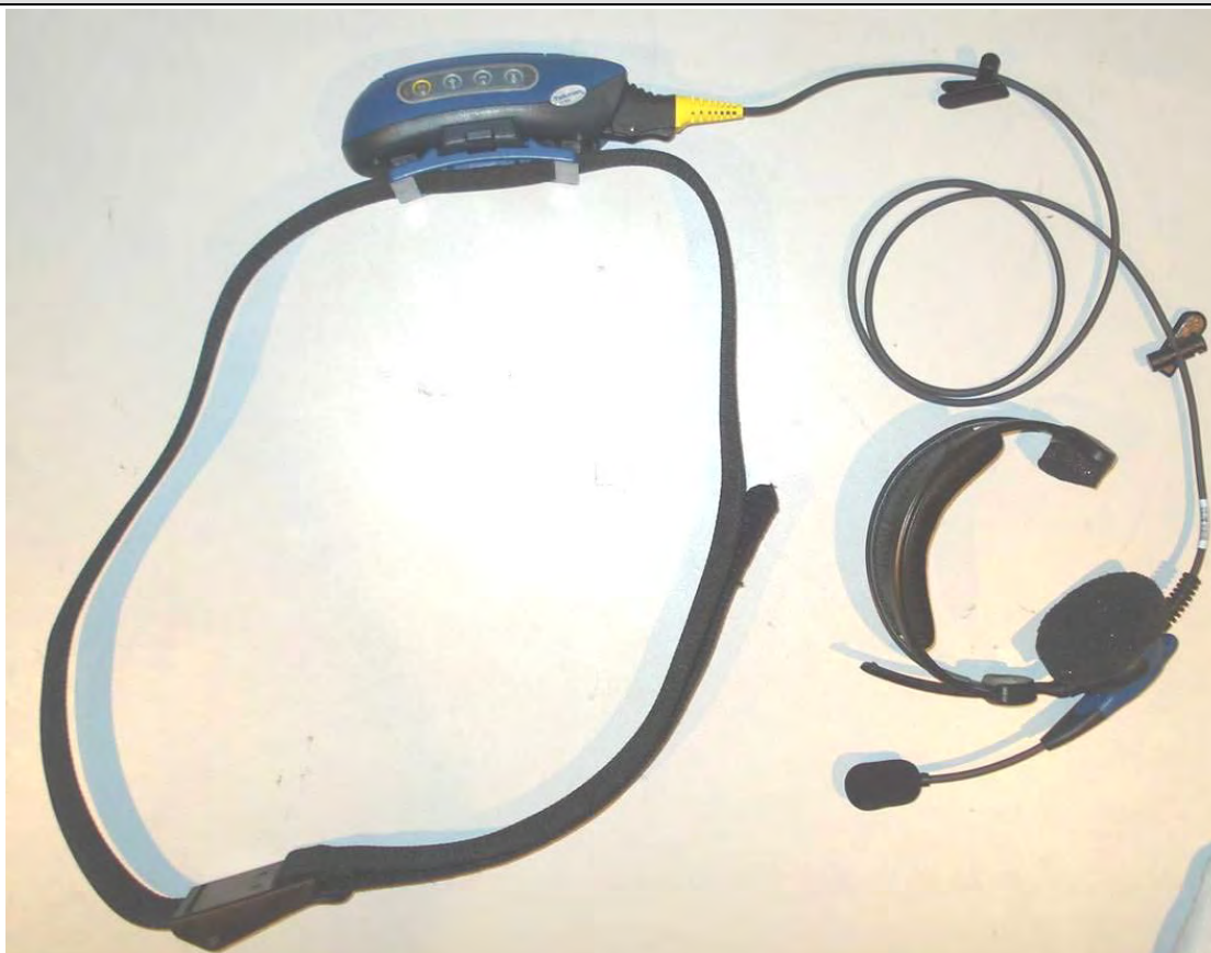
DUT with Headset and Belt-clip/Belt strap accessories
