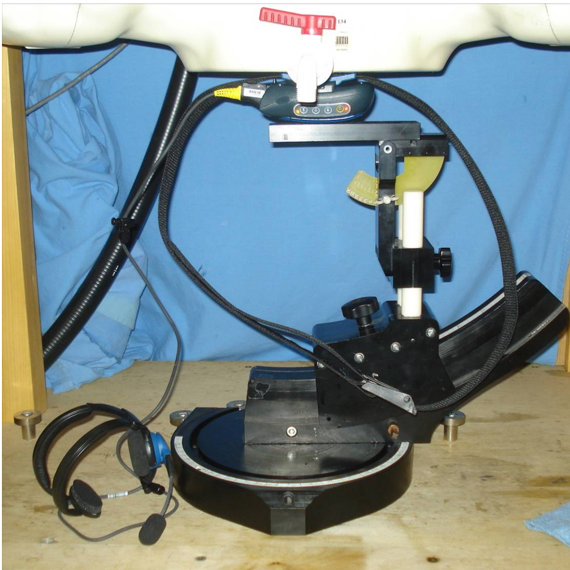
Body-worn Test setup - Belt-clip & Belt-strap Body-worn accessory with Headset-Microphone Audio Accessory
