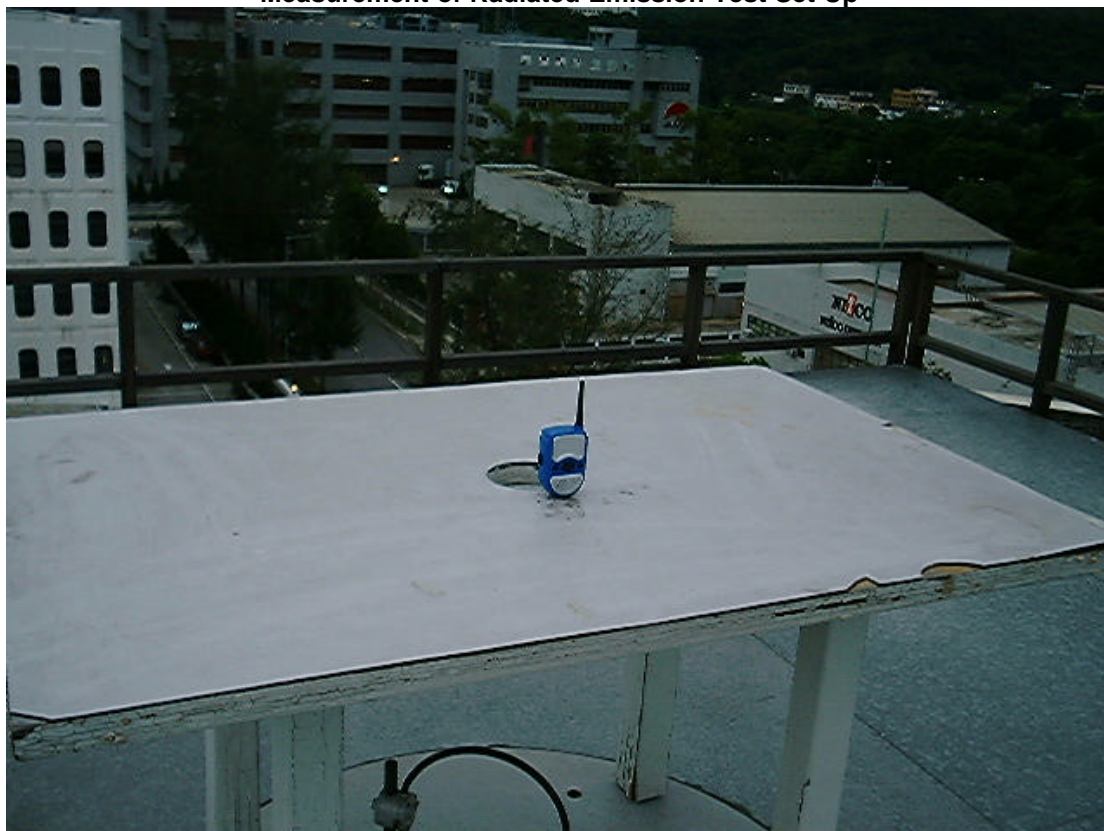
Measurement of Radiated Emission Test Set Up
