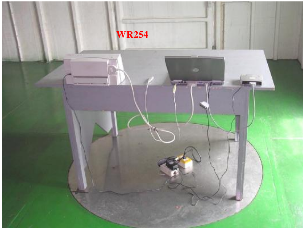
Photo 2: Radiated Emission Test Set-up
