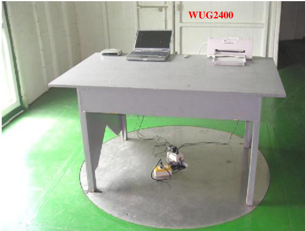
Photo 1: Radiated Emission Test Set-up
