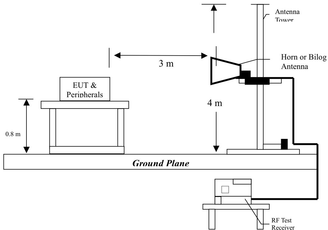
The Diagram below shows the test setup for LAN Function, which is utilized to make these measurements.
