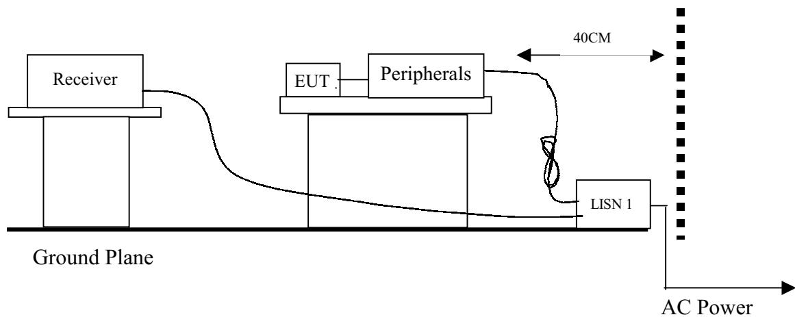
The Diagram below shows the test setup for LAN Function, which is utilized to make these measurements.
