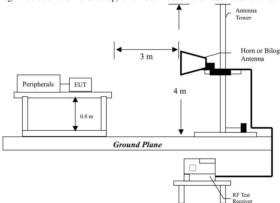
Radiated emission measurements were performed from 30MHz to 25GHz. Spectrum Analyzer Resolution Bandwidth is 100kHz or greater for frequencies 30MHz to 1GHz, 1MHz – for frequencies above 1GHz.
