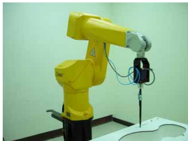
Fig. 5.2 Probe Setup on Robot
