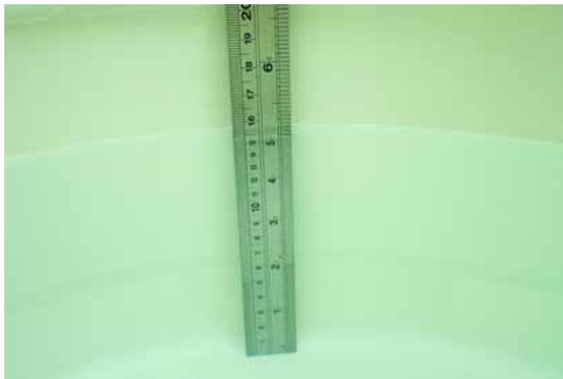
Fig 6.1 Liquid Height from the Bottom of the Phantom Body is 15.2 Centimeters
